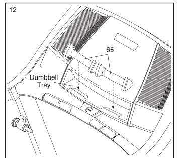
13. Make sure that all parts are properly tightened before you use the treadmill. If there are sheets of plastic on the treadmill decals, remove the plastic. To protect the floor or carpet, place a mat under the treadmill. Note: Extra hardware may be included. Keep the included hex keys in a secure place; one of the hex keys is used to adjust the walking belt (see pages 21 and 22).
