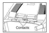
To measure your heart rate, stand on the foot rails and place your hands on the metal contacts—avoid moving your hands. When your pulse is detected, your heart rate will be shown. For the most accurate heart rate reading, continue to hold the contacts for about 15 seconds.
