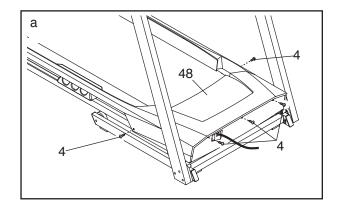
Carefully lift the Motor Hood (48) upward, and then slide it forward and off. Make sure that the Motor Hood does not get caught by the tabs on the sides of the Motor Hood.
