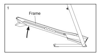
Hold the frame firmly with your right hand. Pull the latch knob to the left and hold it. Raise the frame until the hole in the platform cushion is aligned with the latch pin. Then, slowly release the latch knob; make sure that the latch pin is fully inserted into the platform cushion.
