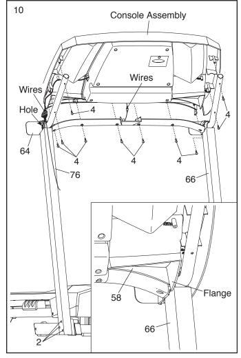
11. Note: There may be two screws (E) preattached to the Left Upright (66). If so, remove and discard the screws.
