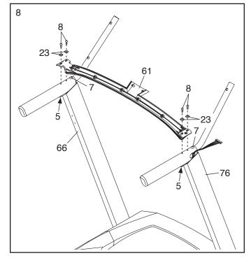
9. With the help of a second person, hold the console assembly near the Right Handrail (64).
