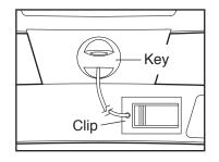
the console. After a moment, the displays will light. IMPORTANT: In an emergency, the key can be pulled from the console, causing the walking belt to slow to a stop. Test the clip by carefully taking a few steps backward; if the key is not pulled from the console, adjust the position of the clip.
